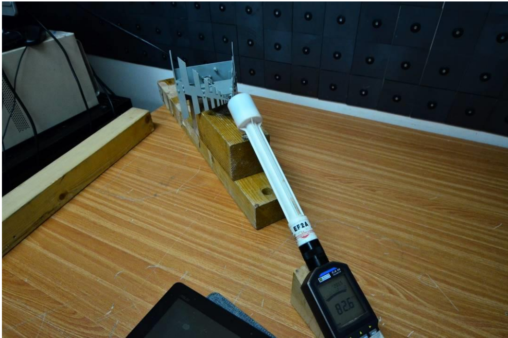
Pic#1: Anti-Radiation universal tablet shield reduction test setup
